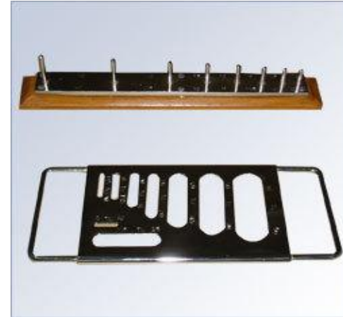
Flakiness & Elongation apparatus
