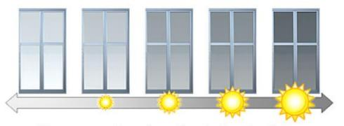
The warmer the glass, the darker the tint. The cooler the glass, the clearer the view.
